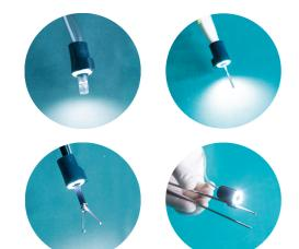
The RUTILIGHT® device is a light ring featuring LED technology which can be adapted to any surgical instrument, in the electro scalpel handle or in any other necessary one in a surgery, without affecting function.
